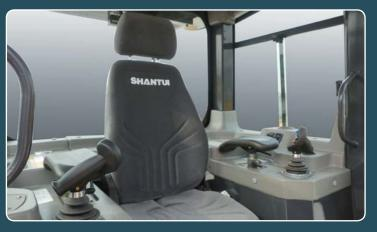
Comfortable fabric, high-back air-suspension seat with adjustable head and back rests are standard. The bottom seat cushion has multi-way adjustments. The seat is for all day operatior comfort for operator support. Optional electric heated seats are available. Separate leather-bolstered arm rests with height and angle adjustments are fitted for operator comfort.
